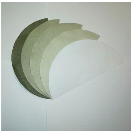
Figure 2 – First experimental results of Brussels sprout paper obtained by Millvision in the Interreg project ‘Growing a Green Future’
