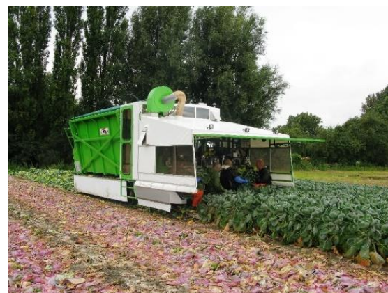
(B) Adapted harvester for bigger production areas (4 rows)
