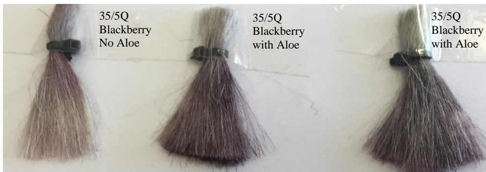
Figure 24 Uptake of Blackberry Extract with and without Aloe Vera – Samples of the dye were reacted with a range of aromatic compounds such as flavonoids which form new complexes - Date: 07.11.17
